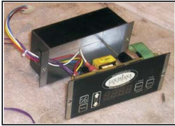
Digi-Que Control Board
